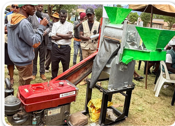
Figure 16: Jacob Mukunuyi, showcasing a combined dehuller and grinding mill (2 in 1) capable of producing super refined mealie-meal in Chimanimani District, Manicaland Province
